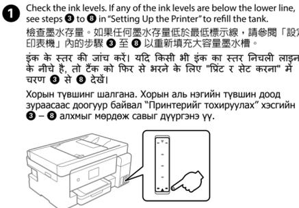
1 Check the ink levels. If any of the ink levels are below the lower line, see steps 3 to 5 in "Setting Up the Printer" to refill the tank.
