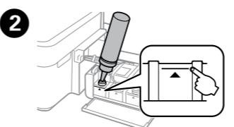
Refer to steps 2 to 9 in section 3 of the front page to refill the tanks to the upper line.
