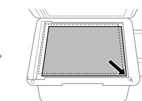
Open the document cover and place your original face-down on the scanner glass. Align the original with the front right corner of the glass.
