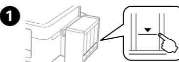
Visually check the ink levels of all ink tanks. If the ink level is below the lower line on the tanks, go to step ② to refill the tanks.
