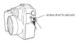
After securely closing the fastener, turn it so that the screw sleeve is covered by the strap, as shown below.
