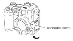
Connect the AV cable to the AV OUT port on the camera as shown below.
