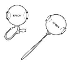
2. Pass the end of the string with the larger loop through the camera strap's triangular fastener as shown below.
