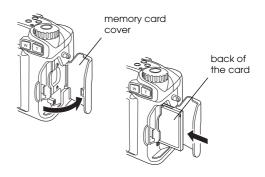
To remove the card, push in the eject button below the memory card slot. Then, remove the card and close the cover.
