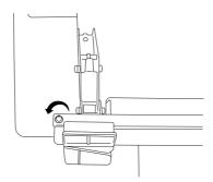
3. Slide and remove the cutter blade unit from the cutter unit, then attach the new cutter blade unit.
