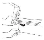
4. Remove the cut paper, and fully slide the cutter blade unit to the left side of the printer.
