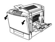
3. Check which color currently appears in the cartridge installation window.
