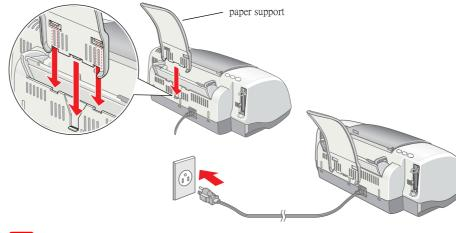
If the printer comes on when you plug in the power cord, turn off the printer by pressing down the O power button until the printer lights go out.
