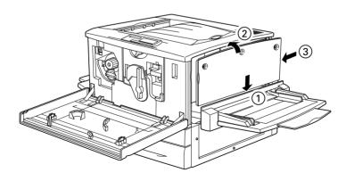
8. Secure the right cover with the screws, then close the front cover and push the paper path unit back into the printer.
