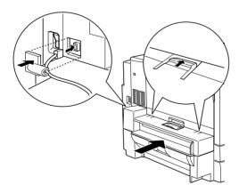
11. Attach the face-up tray onto the Duplex Unit output guide.
