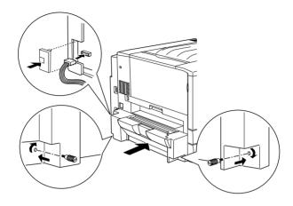
10. Attach the Duplex Unit output guide onto the printer as shown below, then connect the cable to the connector. Finally, conceal the connection using the provided connector cover.
