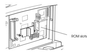
6. Insert the module all the way into slot A or B, making sure that the gold contact side of the module faces up. The X tab on the left of the slot will jut out when the module is inserted correctly.
