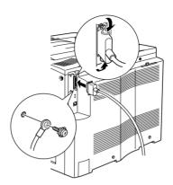
3. Plug the other end of the cable into the computer's parallel interface connector.
