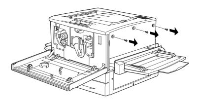
4. Slide the right cover backward, and then remove it by pulling its top as shown below.
