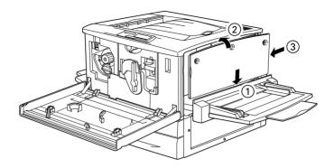
8. Secure the right cover with the screws, then close the front cover and push the paper path unit back into the printer.
