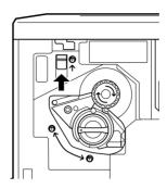
7. Turn the upper knob located just above the cartridge installation window clockwise until it stops. The switch automatically drops down to the lower position and the next empty cartridge slot appears in the cartridge installation window.
