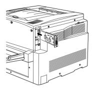
5. Secure the interface card by fastening the retaining screws.
