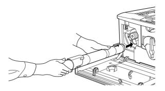
5. Turn the cartridge knob 90 degrees clockwise so that the O symbol on the knob is in the position shown below. By turning the knob, the cartridge is pressed into the slot and installed completely.
