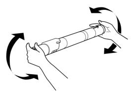
4. Hold the cartridge as shown below, and insert it all the way into the toner cartridge slot until it stops.
