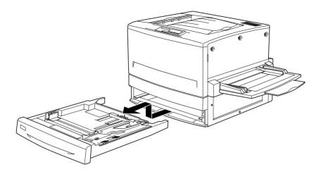
3. Put both legs of the optional 250-Sheet Paper Cassette A3W onto the printer's guide rails, then push the cassette all the way in.
