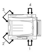
4. Align the corners of the printer and the unit, then lower the printer gently onto the unit so that the three pins on top of the unit fit into the holes on the bottom of the printer.
