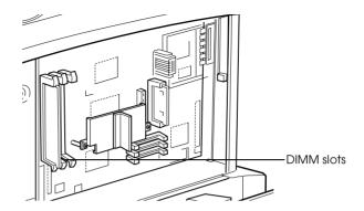
6. Insert the DIMM into either slot, making sure you align it well. The clips on the slot fasten the DIMM when it is inserted correctly.
