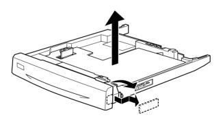
2. Pull out the standard lower cassette and remove it by lifting it up.
