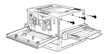
4. Slide the right cover backward, and then remove it by pulling its top as shown below.
