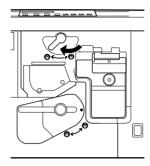
6. Turn the large lever 90 degrees clockwise to an upright position.
