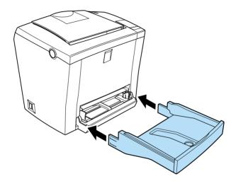
2. Fan a stack of paper (up to 150 sheets), and align the edges by tapping the stack on a flat surface. With the paper's printable side facing upward, place the stack into the tray. Slide the paper guides against the sides of the stack.
