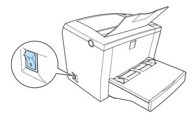
2. Insert the power cord into the back of the printer and plug the other end into a properly grounded electrical outlet.
