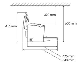
☐ If you install the optional 500-Sheet Lower Paper Cassette Unit, you will need an additional 125 mm (4.9 inches) in height. If you install the optional Face-up Tray, you will need an additional 150 mm (5.9 inches) at the back of the printer.
