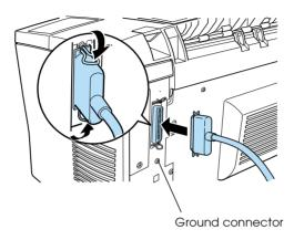
3. Plug the other end of the cable into the computer's parallel interface connector. If there is a ground wire at the computer end of the cable, connect it to the ground connector at the back of the computer.
