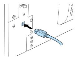
2. Connect the other end of the cable to the computer's USB port.
