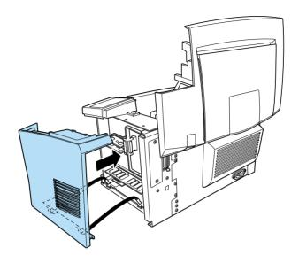
6. Fasten the side cover with the two screws.
