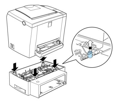
To verify that the 500-Sheet Lower Paper Cassette Unit is correctly installed, print a status sheet. See "Testing the Printer Connection" on page 15.
