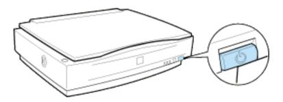
3. Turn on the printer by pressing the (|) side of its power switch.
