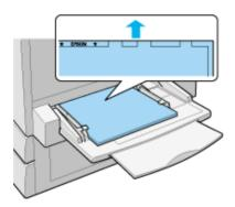
☐ If you attempt to load transparencies in any other way or with the wrong side facing up, the printer ejects the transparency without printing on it to prevent damage to the printer.
