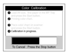
6. When the following screen reappears, remove the first color chart from the scanner, make sure paper is loaded in the MP tray, and press the ♦ start button to print the second color chart.
