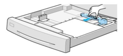
7. Slide the side paper guide so that it points to the size mark that matches the paper loaded.
