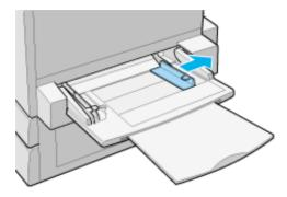
4. Load a stack of the desired media with the printable surface up. Rest the left side of the stack against the left paper guide and slide the right paper guide against the right side of the stack to obtain a snug fit.
