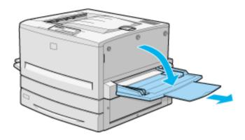
2. If you want to load A3W size paper, lay the left paper guide down. When loading media other than A3W size paper, make sure the guide is standing up.
