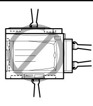
Carry or lift the printer by its correct positions.
