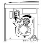
Push the switch up and release it. Turn the knob clockwise until it stops.
