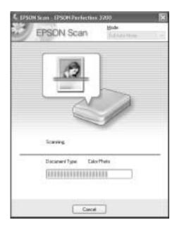
EPSON Scan automatically locates the target images and modifies their skew, and then starts scanning.
