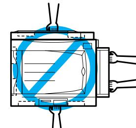
Carry or lift the printer by its correct positions.
