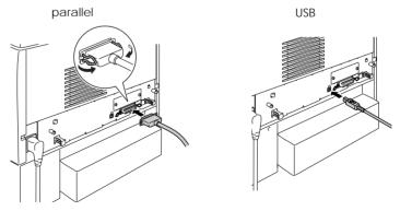
3. Plug the other end of the cable into the computer's parallel or USB interface connector.
