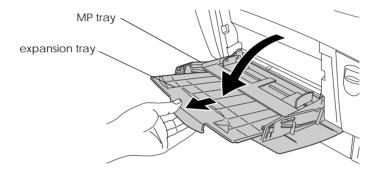
2. Fan a stack of A4 or Letter size paper, then tap it on a flat surface to even the edges. Load the paper in the MP tray.
