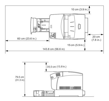
To install and use the optional Large Capacity Paper Unit, you will need an additional 35.2 cm (14.3 in.) to install the unit beneath the printer.
