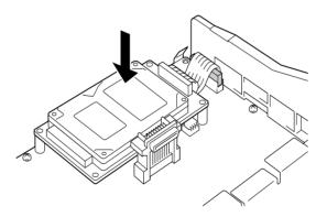
3. Secure the drive with the screws provided.
