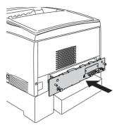
2. Fasten the circuit board tray with the two screws.
