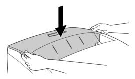
Installing the Photoconductor Unit
