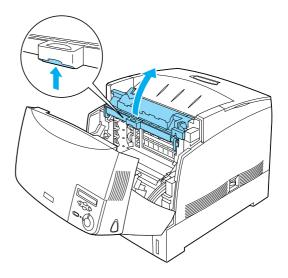
4. Grasp the handle of the photoconductor unit firmly and remove the unit from the printer.
