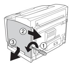
3. Loosen the two screws using a screwdriver. Then hold the tab on the top of the shield cover and remove the cover.
