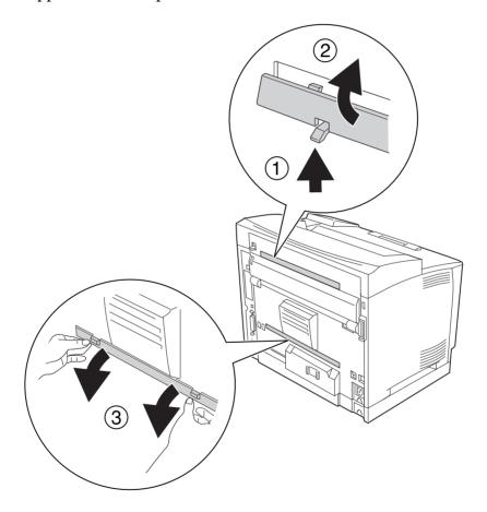
3. Remove the duplex unit connector cover.
