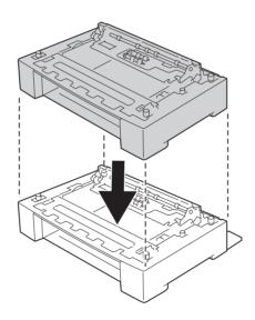
7. Secure the optional paper cassette units with the four fittings. Install two of the four fittings inside on both sides of the optional paper cassette unit and the other two fittings outside on both sides.
