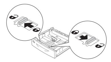
5. Pull out the paper tray to extend the paper cassette and align the arrow marks according to the paper size.
