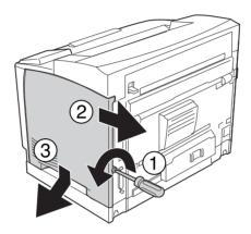
3. Loosen the two screws using a screwdriver. Then hold the tab on the top of the shield cover and remove the cover.
