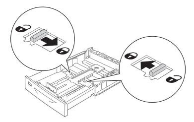
7. Pinch the knobs and slide the paper guide to accommodate the paper you are loading.
