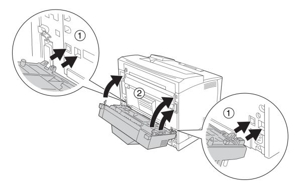
5. Secure the Duplex Unit with the two screws.
