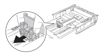
8. Load a stack of the desired paper on the center of the paper cassette with the printable surface facing up.
