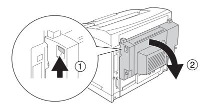
2. Open the paper holder by pulling down the lever with a black star on it.
