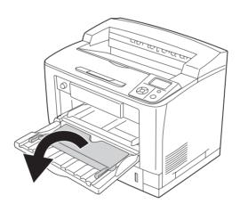
3. Load a stack of the desired paper with the printable surface facing up. Then slide the paper guides to get a snug fit.
