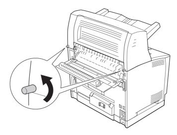
4. Hold up the Stacker and remove the right and left tabs from the holes of the top of the printer.
