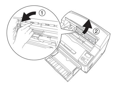
6. Reinstall the imaging cartridge.
