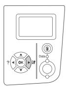
3. Confirm that the information about the installed options is correct. If the options are installed correctly, they appear under Hardware Configuration. If the options are not listed, try reinstalling them.
