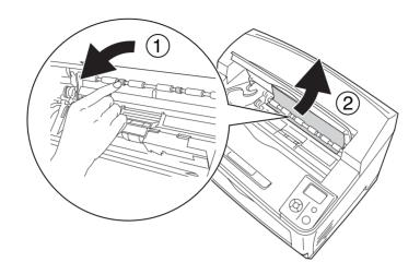
8. Reinstall the imaging cartridge.
