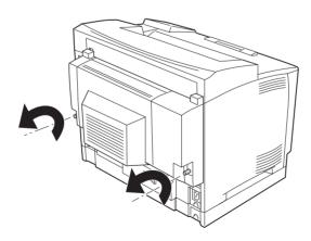
3. Press the unlock button to unlock the hooks, then remove the Duplex Unit from the printer.
