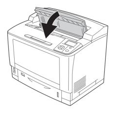
Note: When the optional Stacker is installed, close cover A first, then lower the stacker.
