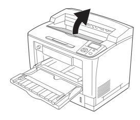
Note: When the optional Stacker is installed, raise the stacker first, then open cover A.
