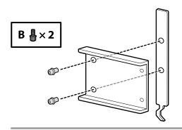
Give the screws shown in the figure a couple of turns to fasten the parts temporarily. The items in the following steps can not be attached if the screws are too tight.
