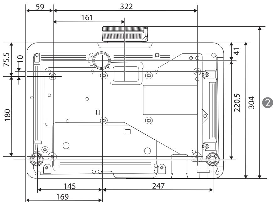
② EB-L735U/EB-L730U/EB-L720U/EB-L630U/EB-L530U: 339 mm
