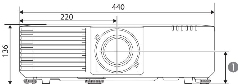
① Distance from center of lens to suspension bracket fixing point : 74 mm
