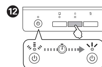
Press **△** for **3 seconds** until **○** starts flashing. Charging ink takes about 22 minutes. Wait until the light stays on.
