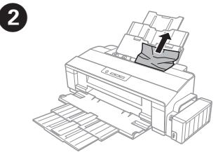
Close the printer cover. If the jammed paper remains near the rear paper feed, carefully remove the paper.
