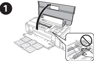
Open the printer cover and remove all of the paper inside, including any torn pieces.
