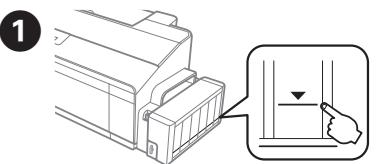
Check the ink levels. If an ink level is below the lower line, refill the ink.
