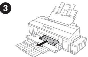
If the jammed paper remains inside the output tray, carefully remove the paper.
