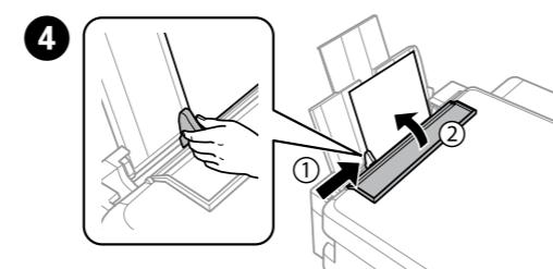
Slide the edge guide against the paper, then close the feeder guard.
