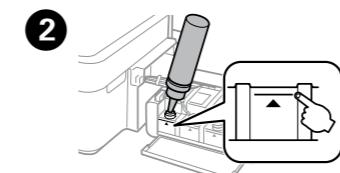
Refer to steps ② to ⑨ in section 3 of the front page to refill the tanks to the upper line.
