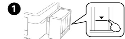
Visually check the ink levels of all ink tanks. If the ink level is below the lower line on the tanks, go to step ② to refill the tanks.
