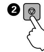
Run the print head cleaning. Hold down ⚡ for 3 seconds until the power light starts flashing. The cleaning uses some ink from all tanks, so run the cleaning only if print quality declines on your prints.
