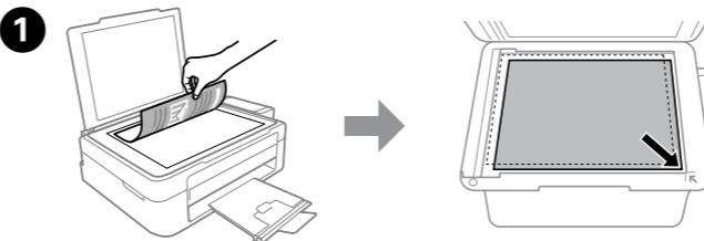
Open the document cover and place your original face-down on the scanner glass. Align the original with the front right corner of the glass.
