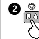
Run the print head cleaning. Hold down for 3 seconds until the power light starts flashing.
