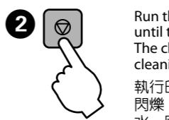
Run the print head cleaning. Hold down ◇ for 3 seconds until the power light starts flashing. The cleaning uses some ink from all tanks, so run the cleaning only if print quality declines on your prints.
