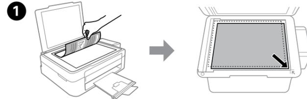
Open the document cover and place your original face-down on the scanner glass. Align the original with the front right corner of the glass.
