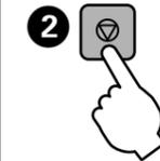
Run print head cleaning until all lines are printed completely. Hold down for 3 seconds until the power light starts flashing. Print head cleaning starts. 執行印字頭清潔，直到所有線條均完整列印為止。按住 鍵 3 秒，直到電源燈號開始閃爍。印字頭清潔開始。
