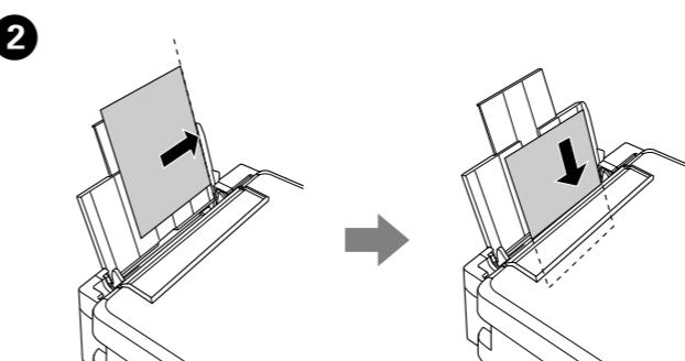
Load paper with the printable side face-up against the right side of the sheet feeder. 將紙張的列印面朝上，靠齊自動進紙槽的右側放入。
