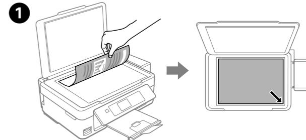
Open the document cover and place your original face-down on the scanner glass. Align the original with the front right corner of the glass.
