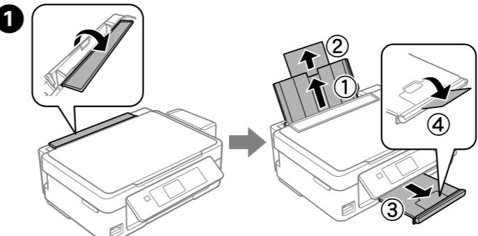
Flip the feeder guard, and then slide out the paper support and the output tray. 翻開進紙槽護蓋，然後滑出紙張支撐板及出紙托盤。
