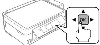
When the message of seeing the setup manual is displayed, press **OK** for **3 seconds**.
