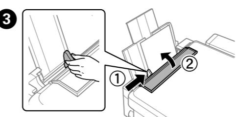
Slide the edge guide against the paper, and flip the guard back. 靠著紙張滑動邊緣定位器，然後翻回護蓋。
