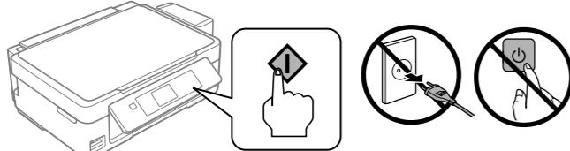
Confirm that the tanks are filled with ink, and then press **◊** to start charging ink. Charging ink takes about 20 minutes.
