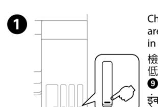
1 Check the ink levels. If any of the ink levels are below the lower line, see steps ① to ⑨ in section 2 to refill the tank.
