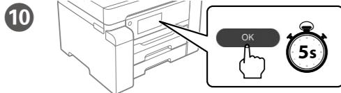
When the message of seeing Start Here is displayed, press **OK** for **5 seconds**.
