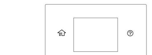
Displays the home screen. You can select other menus such as scan or printer settings. The copy menu is displayed when you turn on the printer or when it returns from sleep mode.
