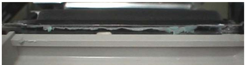
Adhesive adheres on cutter blade
