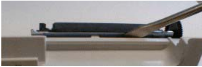
Adhesive being removed with flat-blade screwdriver
