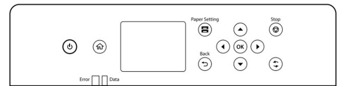
Turns the printer on or off. Unplug the power cord when the power light is off.
