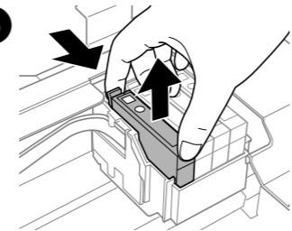
Squeeze the tab on the ink cartridge and lift it out.
