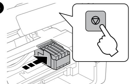
Press again to move the print head to the ink cartridge replacement position.
