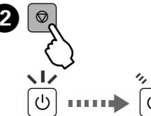
Run the print head cleaning. Hold down for 3 seconds until the power light starts flashing.
