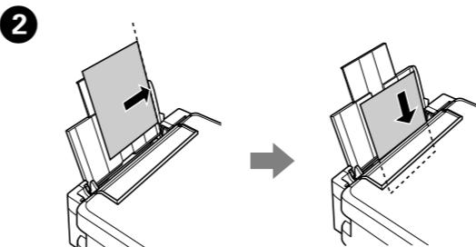
Load paper with the printable side face-up against the right side of the sheet feeder.
