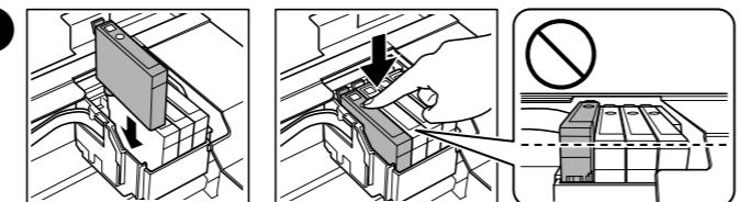
Insert the new ink cartridge and press it down firmly.
