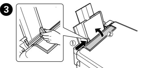
Slide the edge guide against the paper, and flip the guard back.
