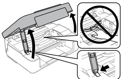
Open the scanner unit and press . The print head moves. If the print head does not move, hold down for 6 seconds or more until it moves.
