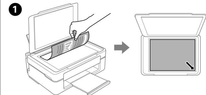
Open the document cover and place your original face-down on the scanner glass. Align the original with the front right corner of the glass.
