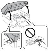
Never touch the ink cartridges while the print head is moving. 當印字頭移動時,切勿碰觸墨水匣。
